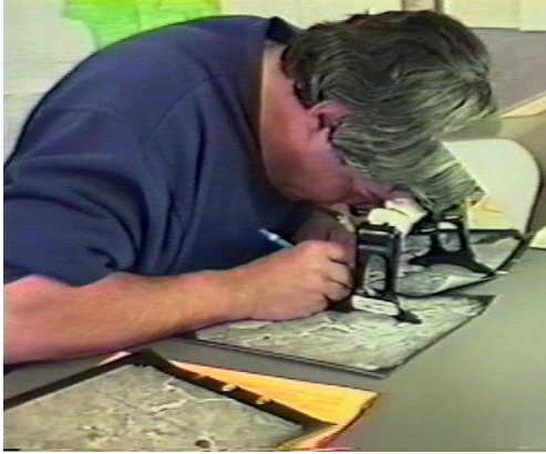
Photo Interpretation Specialist Dave Johnston delineating forest stands on a stereo-pair of 1:20,000 scale aerial photographs with the aid of a Pocket Stereoscope circa 1994
